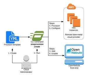
All operations with the provision and physical resources are performed only with the command line tool oneprovision. Create a new provision, manage (reboot, reset, power off, resume) the existing provisions, and delete the provision at the end.
