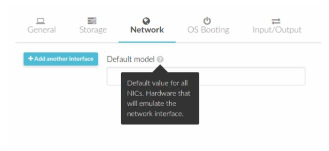
This networking customization can be disabled for each Template. The users instantiating the Template will not be able to add, remove, or customize set NICs set by the Template owner.
