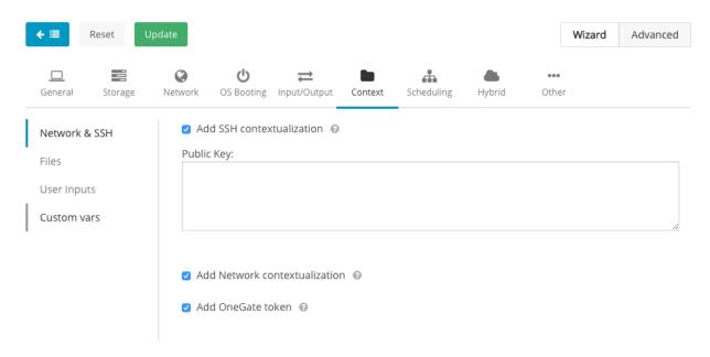
When this Template is instantiated, OpenNebula will automatically add the ONEGATE\_ENDPOINT context variable, and a token.txt will be placed in the context cdrom. This token.txt file is only accessible from inside the VM.
