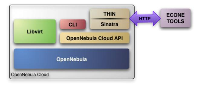
The current implementation includes the basic routines to use a Cloud, namely: image upload and registration, and the VM run, describe and terminate operations. The following sections explain you how to install and configure the EC2 Query web service on top of a running OpenNebula cloud.
