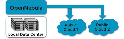
OpenNebula's approach to cloud bursting is based on the transparency to both end users and cloud administrators to use and maintain the cloud bursting functionality. The **transparency to cloud administrators** comes from the fact that a AWS EC2 region or an Azure location is modeled as any other host (albeit of potentially a much bigger capacity), so the scheduler can place VMs in the external cloud as it will do in any other local host.
