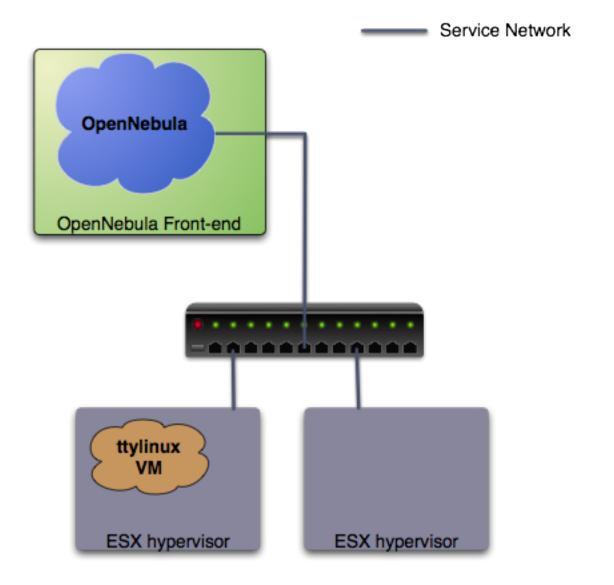
In this guide it is assumed that at least two physical servers are available, one to host the OpenNebula front-end and one to be used as a ESX virtualization node (this is the one you need to configure in the following section). The figure depicts one more ESX host, to show that the pilot cloud is ready to grow just by adding more virtualization nodes.
