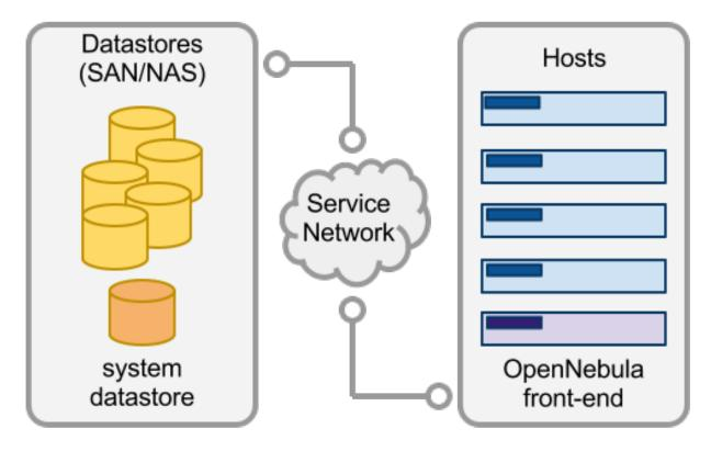
When a VM is deployed the Images are *transferred* from the Datastore to the hosts. Depending on the actual storage technology used it can mean a real transfer, a symbolic link or setting up an LVM volume.
