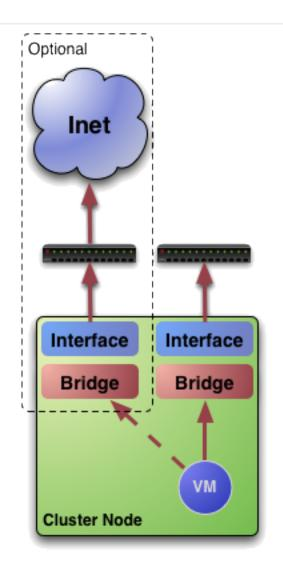
A network connection is needed by the OpenNebula front-end daemons to access the hosts to manage and monitor the hypervisors; and move image files. It is highly recommended to install a dedicated network for this purpose.
