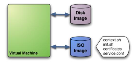
In this example we see a Virtual Machine with two associated disks. The Disk Image holds the filesystem where the Operating System will run from. The ISO image has the contextualization for that VM:
